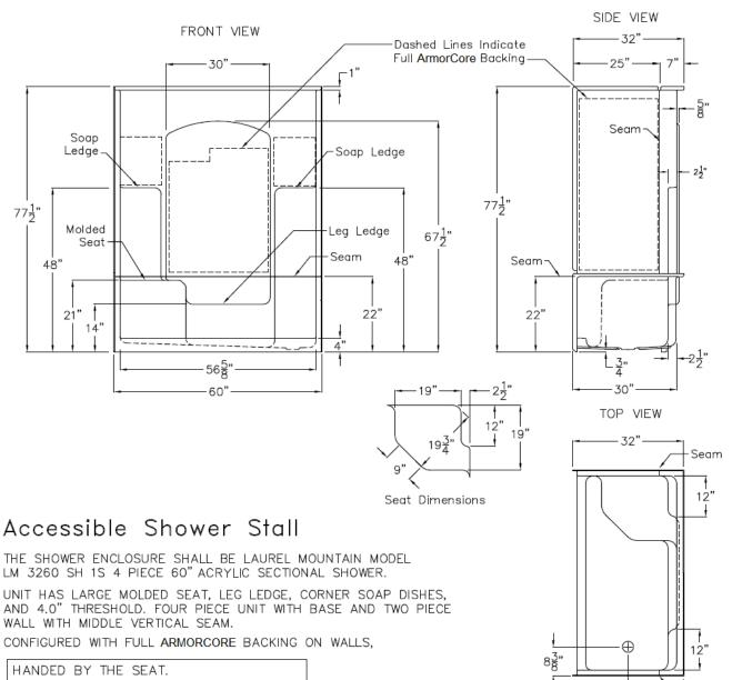
LEFT HAND SEAT HAS RIGHT HAND DRAIN RIGHT HAND SEAT HAS LEFT HAND DRAIN
